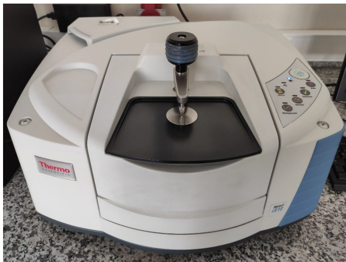
Figure 4.8 Image of the used FTIR device having ATR apparatus (Personal archive, 2021)
