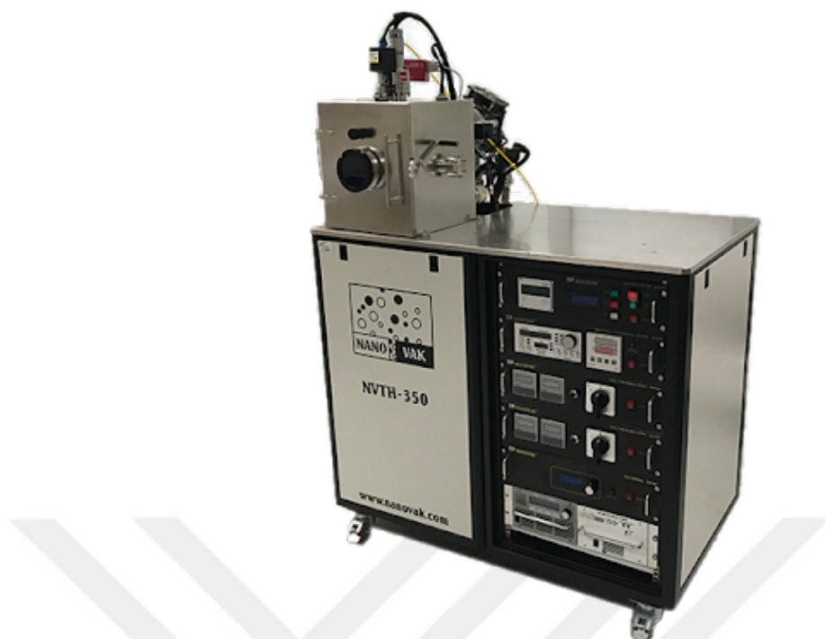
Figure 4.2 RF Magnetron Sputtering device (Personal archive, 2020)
