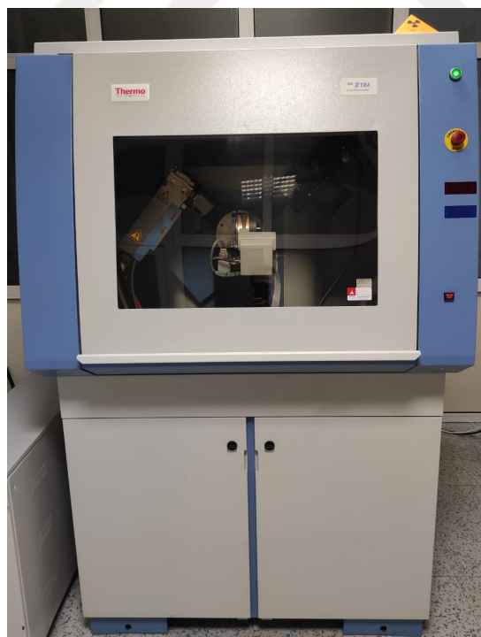
Figure 4.4 X-Ray Diffractometer, Thermoscientific ARL X'TRA (Personal archive, 2020)
