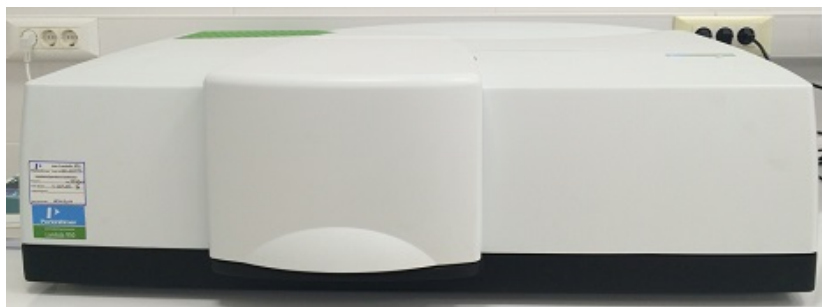
Figure 4.7 Perkin Elmer, Lambda 950 UV/VIS/NIR spectrophotometer device (Personal archive, 2020)
