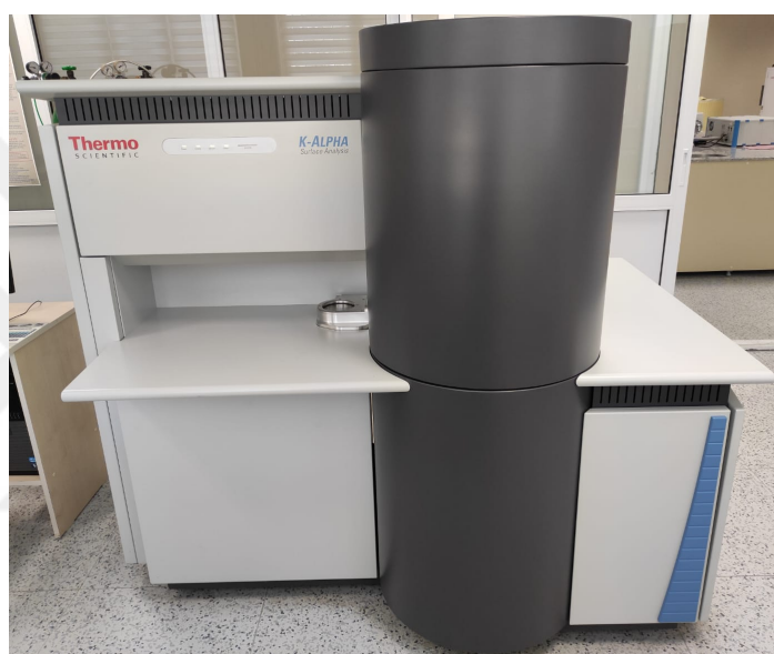
Figure 4.6 Thermo Scientific K-Alpha XPS device (Personal archive, 2020)
