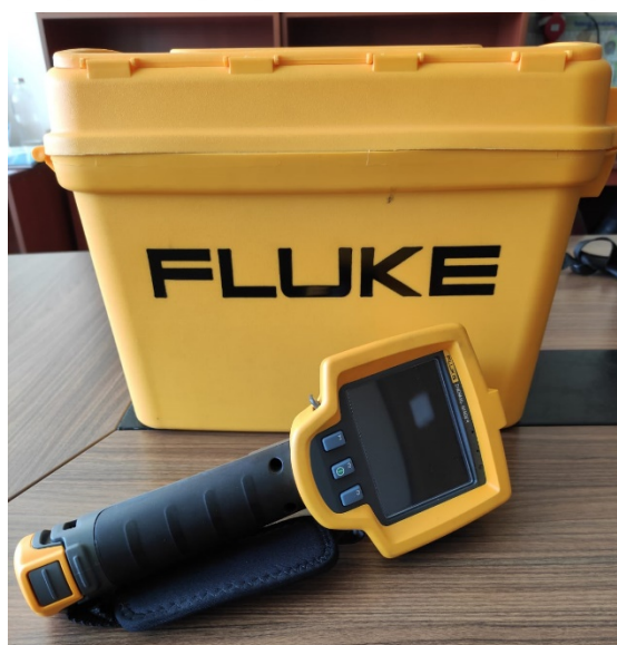
Figure 4.9 Fluke, Ti27 thermal camera (Personal archive, 2020)
