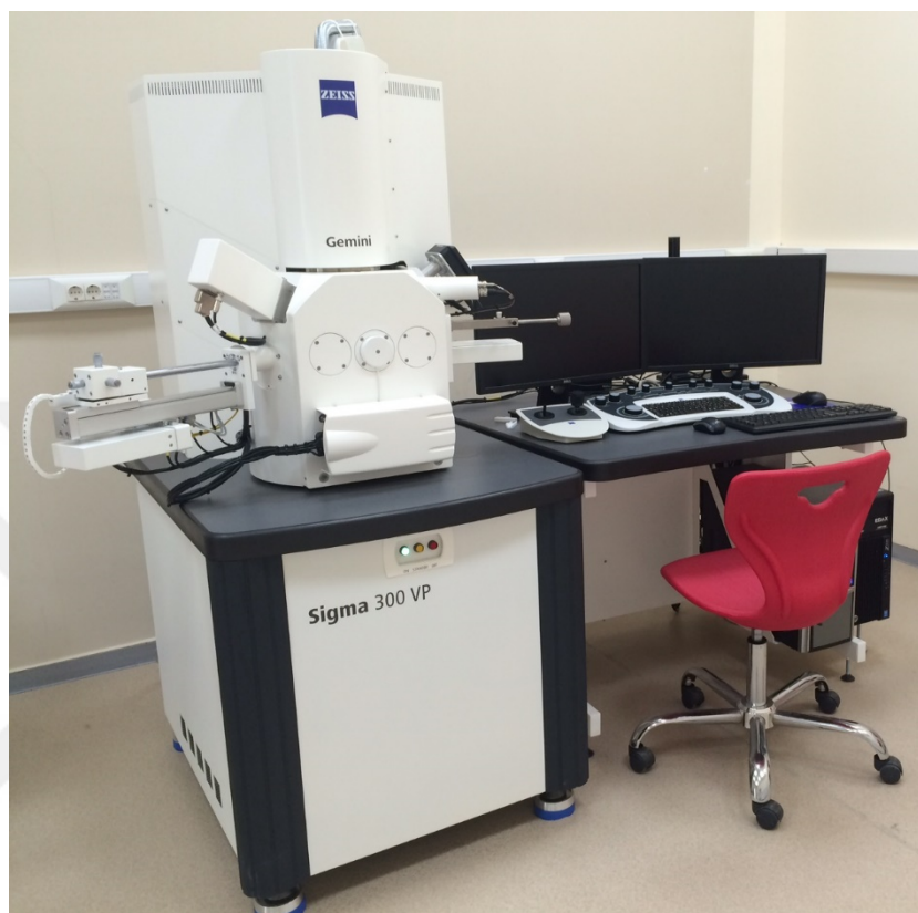
Figure 4.5 Zeiss Gemini model SEM device (Personal archive, 2020)
