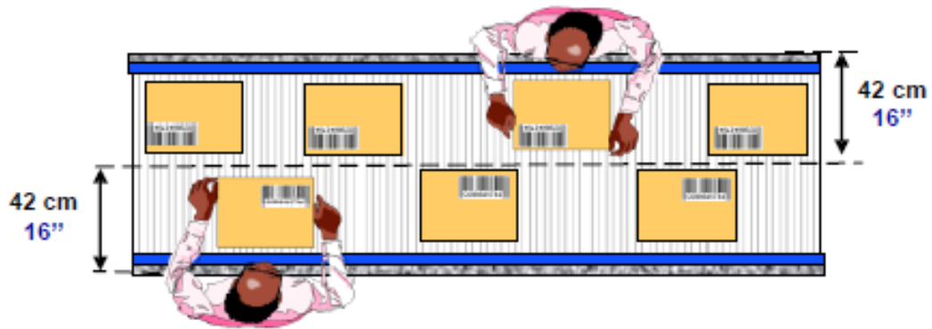
Figure 1.1 The proper distance of reach to avoid MSDs due to prolonged and repetitive leaning (Schneider Electric Magazine, 2014)
