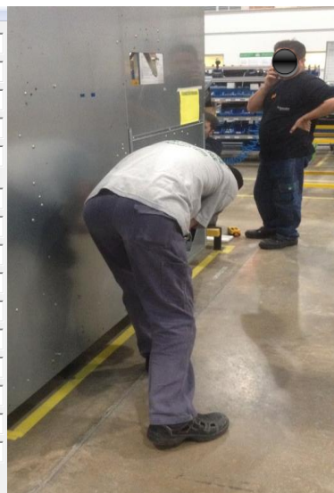
Figure 3.30 REBA score-5 in the Door and Roof Assembly Section (Personal archive, 2019)
