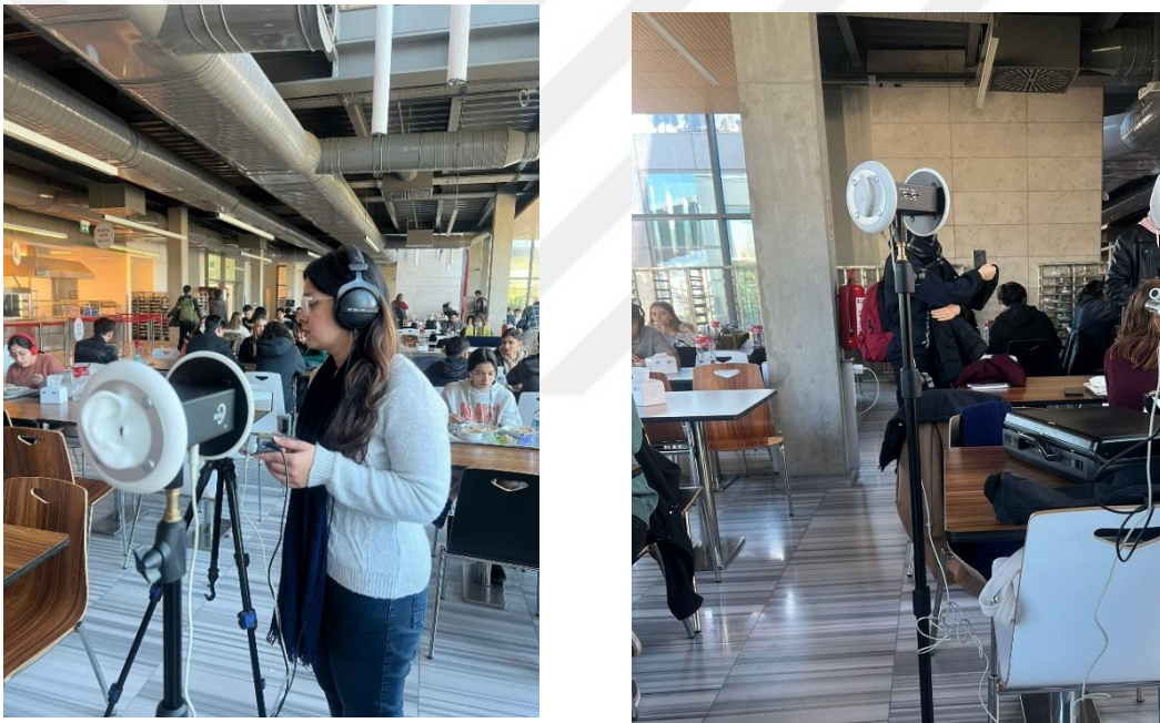
Figure 4: Figure 4: Bruel & Kjaer 2230 sound level meter, ZoomH4 sound recorder & Binaural microphone.
