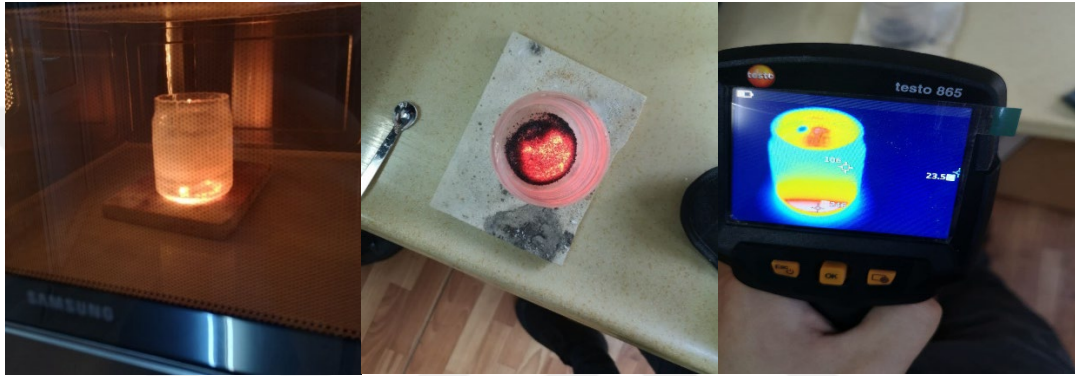
Figure 4.26. Photographs of the ore ( -1+0.500 mm) exposed to microwave treatment
