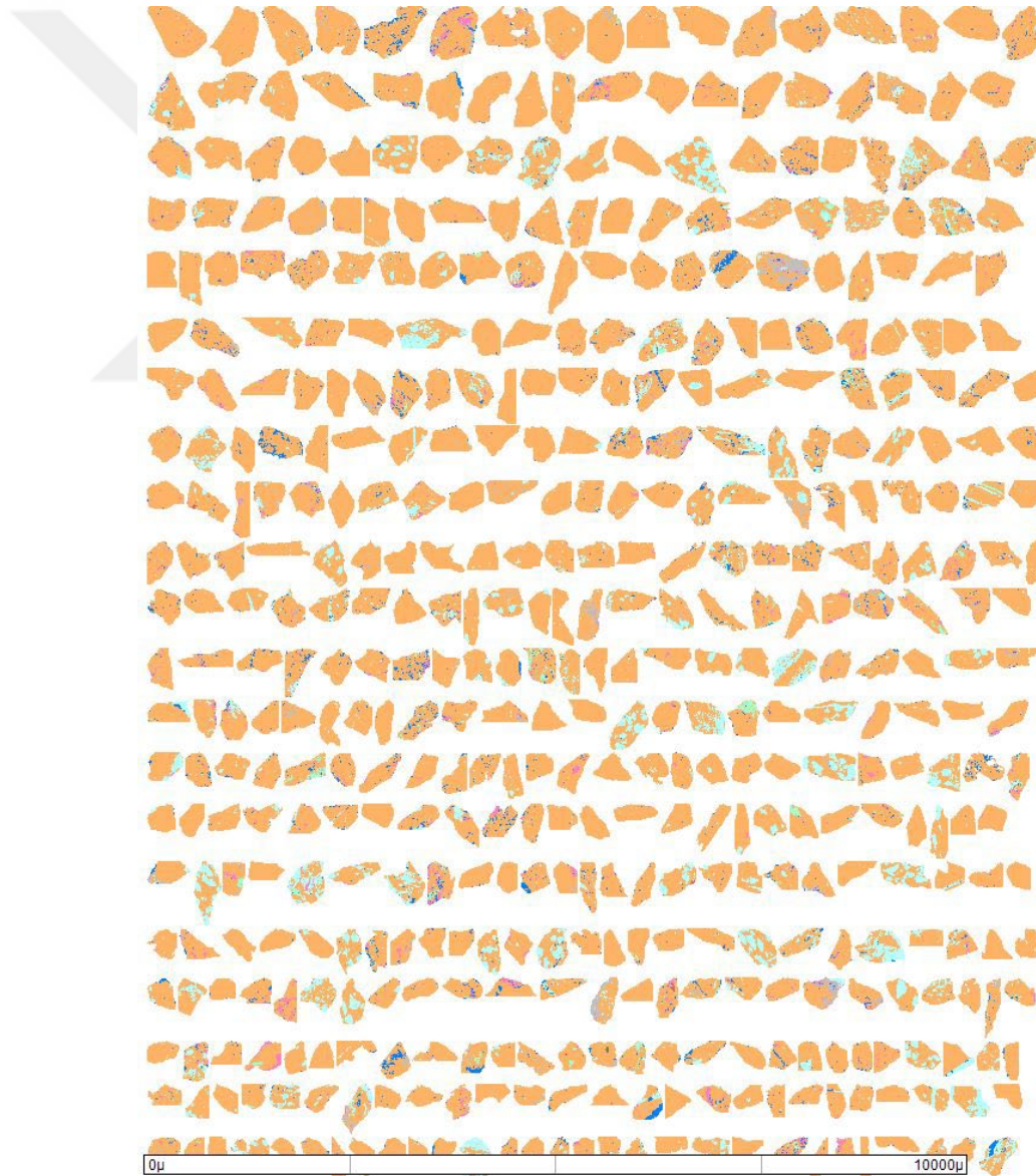
Figure 4.1. MLA classified images showing iron-oxide in the sample
