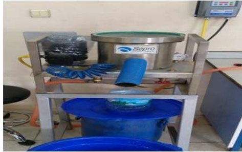
Figure 3.9. Falcon separator used in the study.
