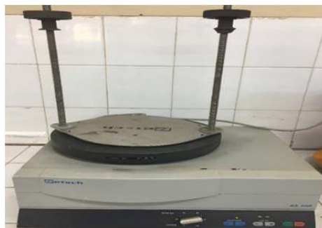
Figure 3.4. RETSCH Sieve Shaker AS 200 used in experiments.
