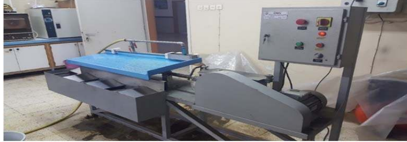
Figure 3.8. Wilfley laboratory type shaking table used in experiments.
