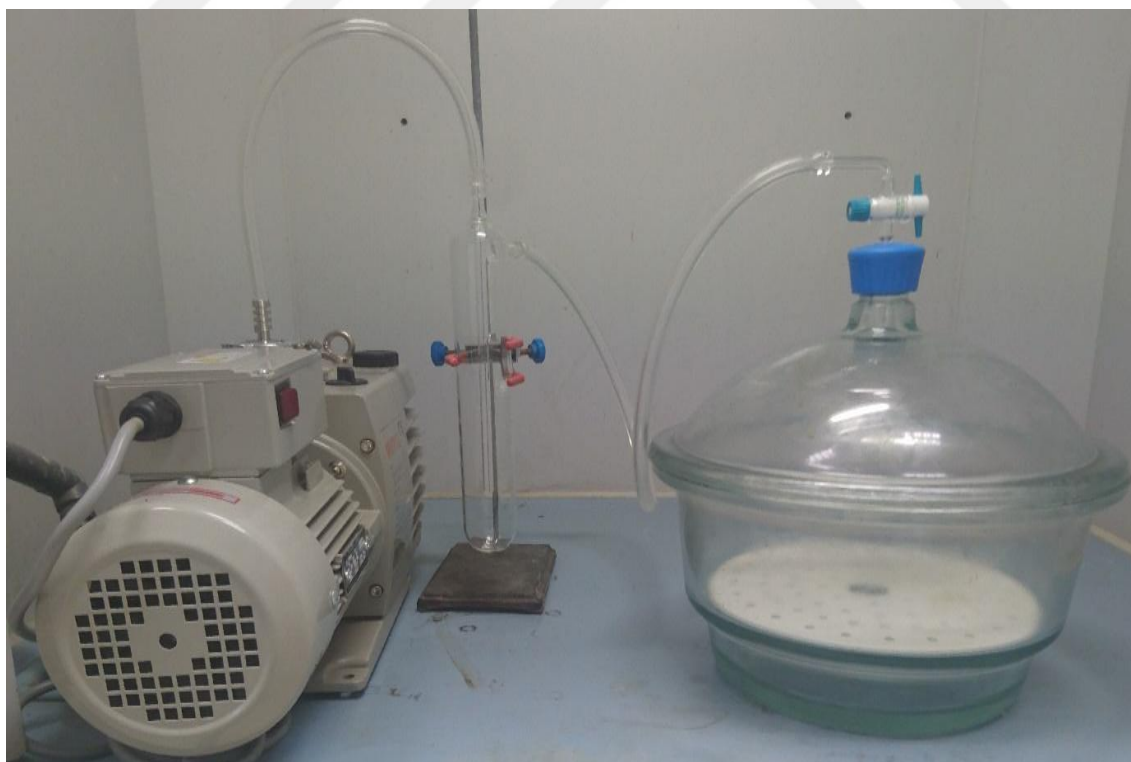
Figure 2.1 The setup for the vacuum-drying in the desiccator (on the right) of the lyophilization of polymer samples with a vacuum pump (on the left).
