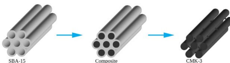
Figure 1. 1. Schematic representation of hard templating method (HTM). Adapted with permission from license No. 5562470501392, ELSEVIER, 2013.
