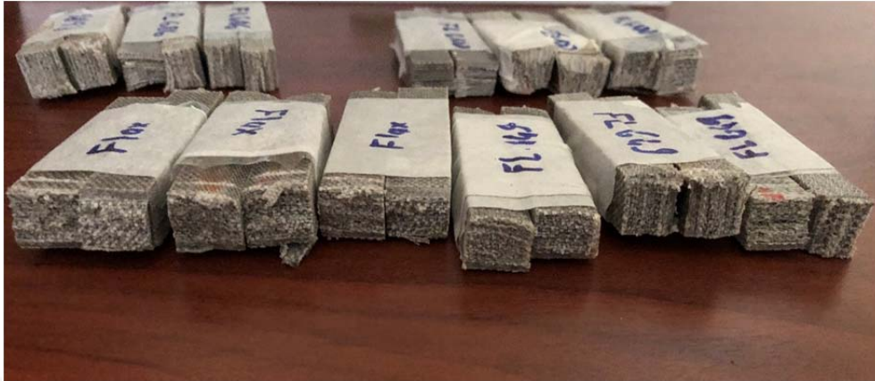
Figure 4.25. Fracture zone sections of materials after impact testing
