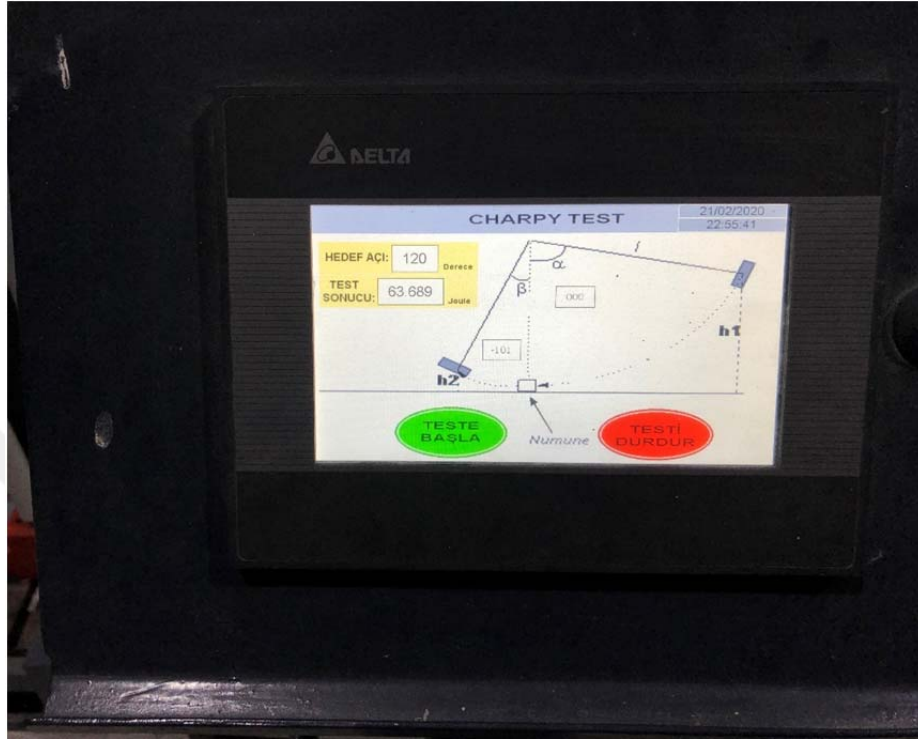
Figure 3.35. Data screen of Charpy impact test machine
