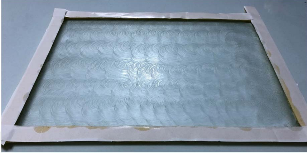
Figure 3.19. Mold release wax applied surface
