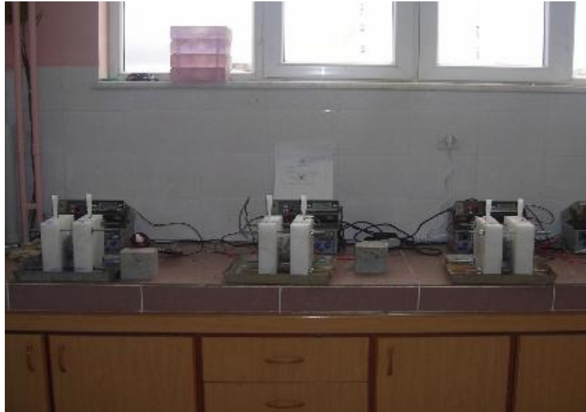
Figure 3.7 Rapid chloride permeability test
