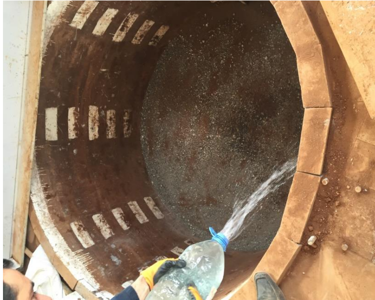
Figure 3.12 Spreading of water for compaction in plate load box
