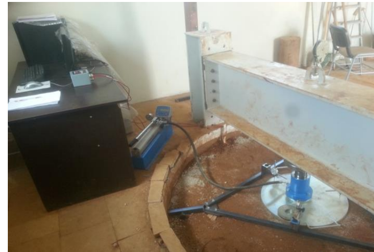
Figure 3.18 Schematic view of the test setup, loading and sampling system with the actual box model and plate load apparatus
