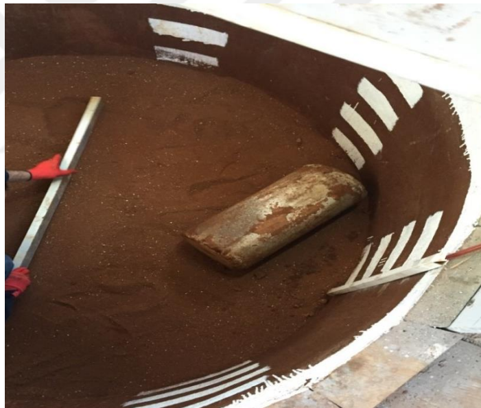
Figure 3.10 Mixing of dry CDMs with dry clay for compaction in plate load box (a) CBPs, (b) DAPs, and (c) CCPs
