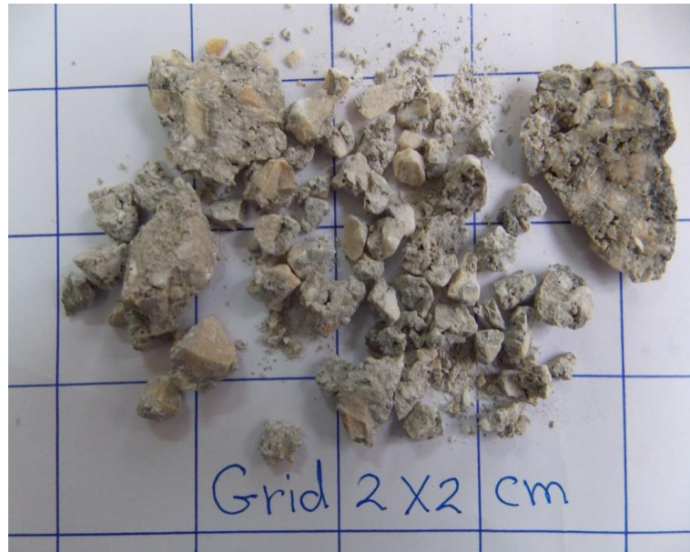
Figure 3.4 Pictures of CDMs used in CBR test (a) crushed brick pieces, (b) dump asphalt pieces, and (c) crushed concrete pieces
