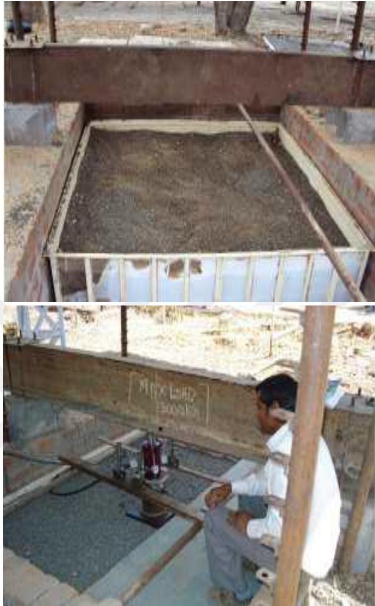
Figure 2.10 Pictures of plate load test on granular layered soils (Sanjeev et al., 2013)
