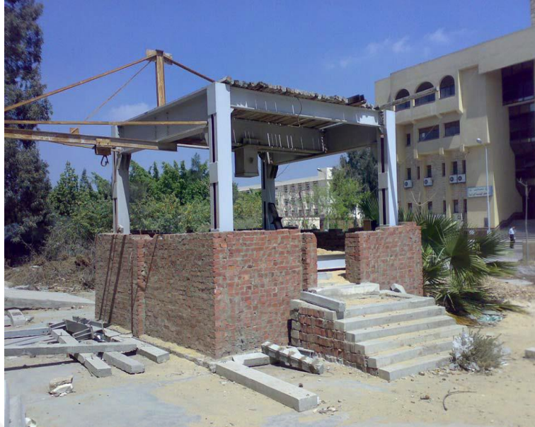
Figure 2.11 Effect of foundation dimensions and shape using box model with a frame (Abd elsamee, 2013)
