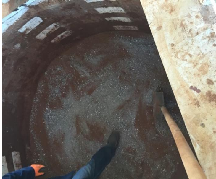
Figure 3.10 Mixing of dry CDMs with dry clay for compaction in plate load box (a) CBPs, (b) DAPs, and (c) CCPs
