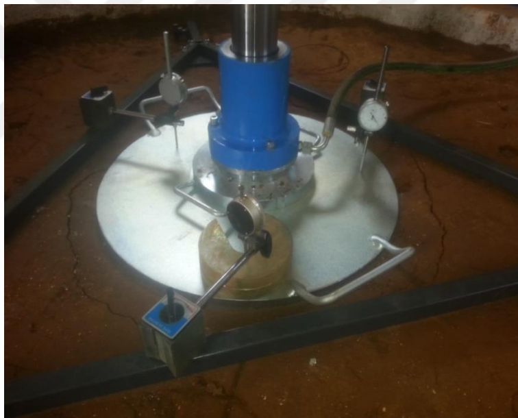
Figure 3.19 Picture showing the location of the bearing plate and strain gauges used for plate load test
