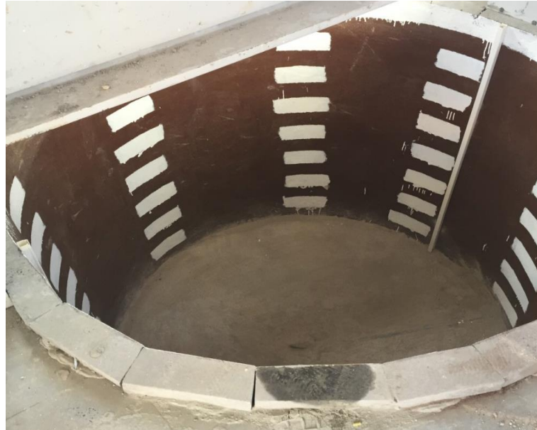
Figure 3.9 Picture of preparing of the box by painting for soil compaction
