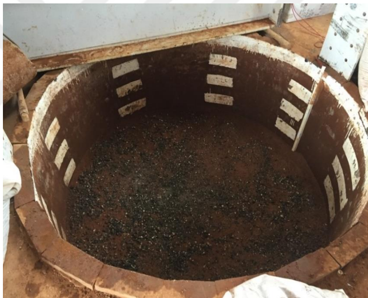
Figure 3.13 Clay-CDMs mixtures just before compaction in plate load box
