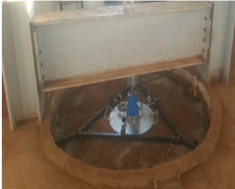
Figure 3.19 Picture showing the location of the bearing plate and strain gauges used for plate load test
