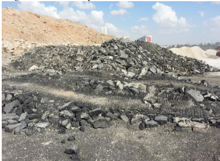
Figure 3.3 Picture of pile of old pavement asphalt
