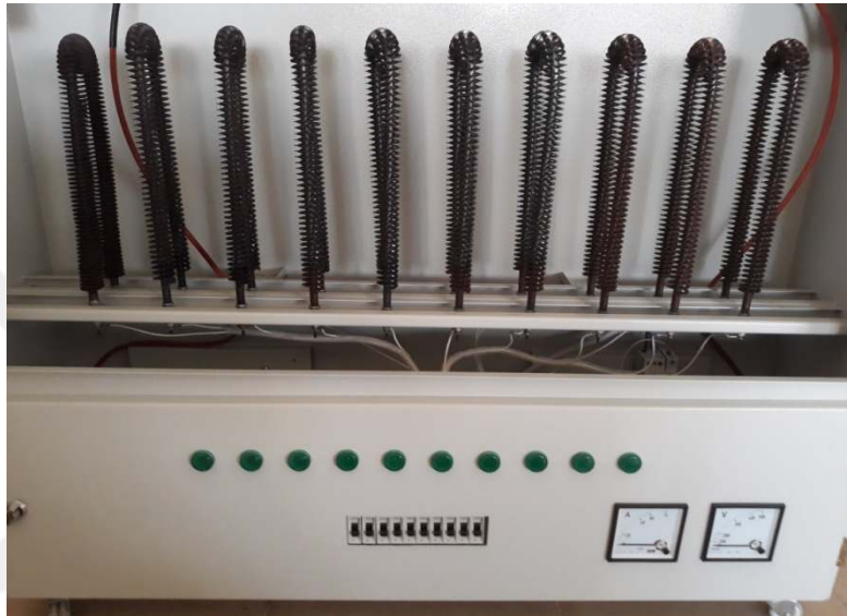
Figure 5.21. Electric loading system
