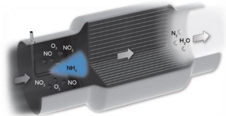
Figure 3.2. Selective catalytic reduction system (Anar and Bayram, 2018)
