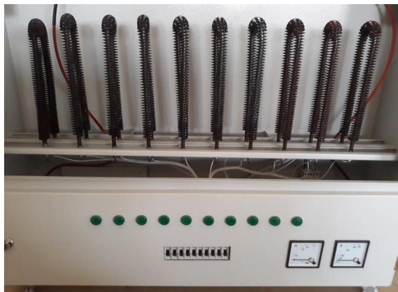
Figure 5.14. Electric loading system
