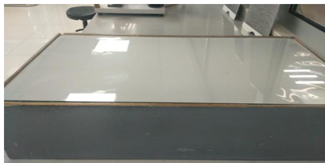
Figure 3.6. Carding Neps Control Light Box
