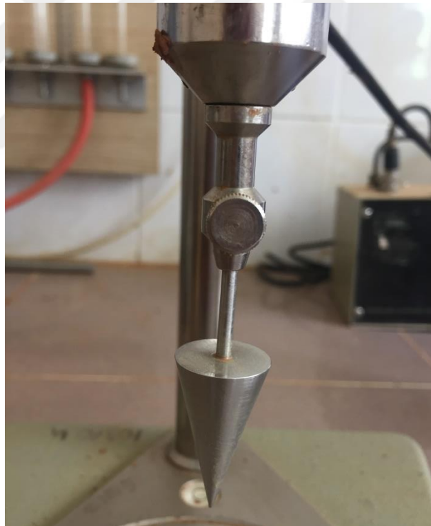
Figure 3.18 The stainless steel penetration cone
