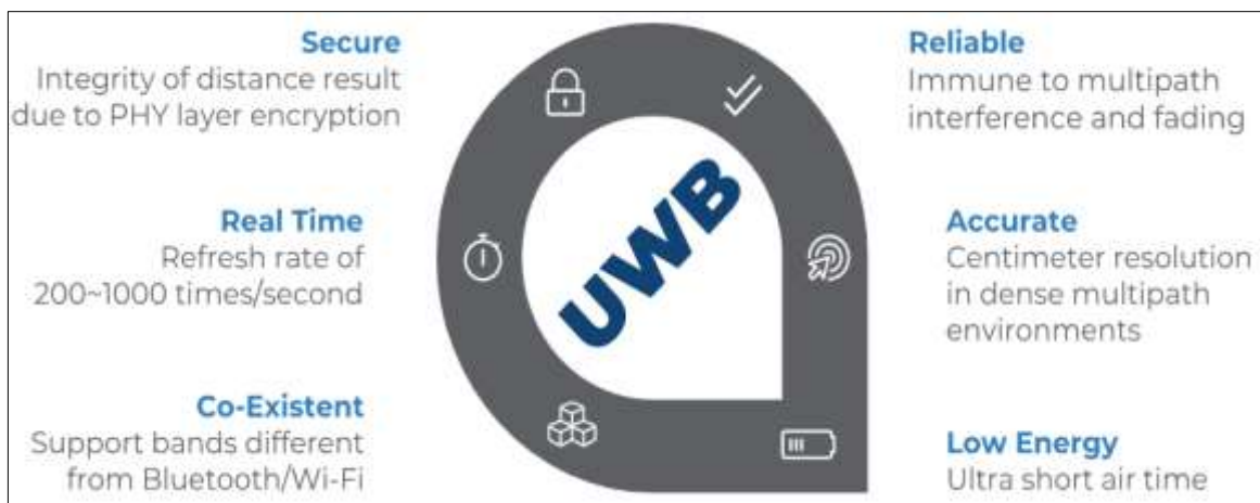
Figure 1.3: UWB Technology Properties.
