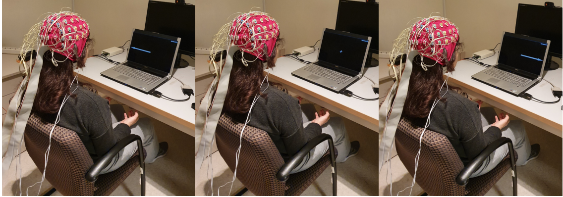
Figure 6.1: A user attending a session of the two-class motor imagery experiment that generated the SPIS MI-BCI dataset.
