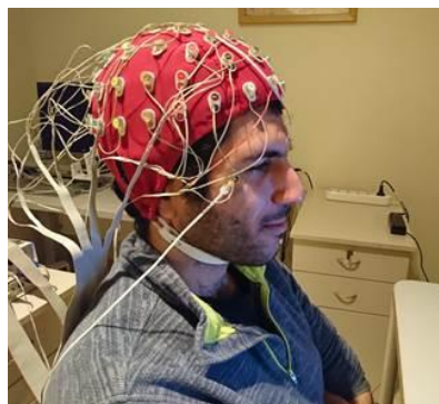
Figure 3.1: A user wearing the 64-channel Biosemi headset (Biosemi Inc., Amsterdam, the Netherlands) and 3 surface EOG electrodes.
