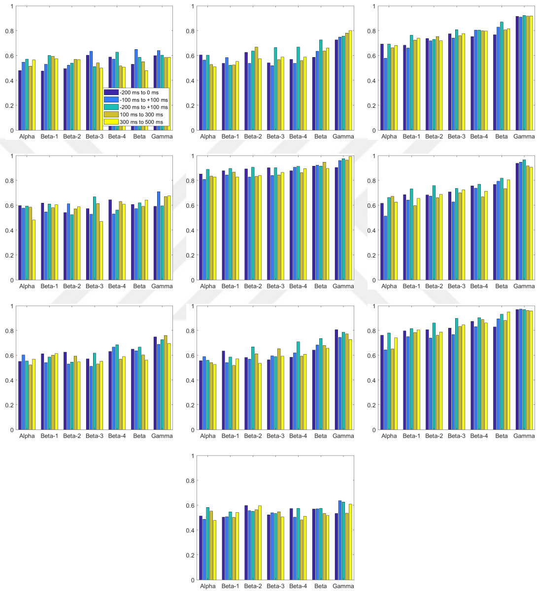
Figure 4.7: AUC of precision-recall curves for within-subject drowsy-vs-alert state detection using 5 time intervals and 7 PLV bands.
