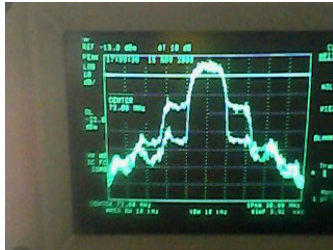
Figure 5.17: Spectrum of PA Output Using Predistortion at High Input Power
