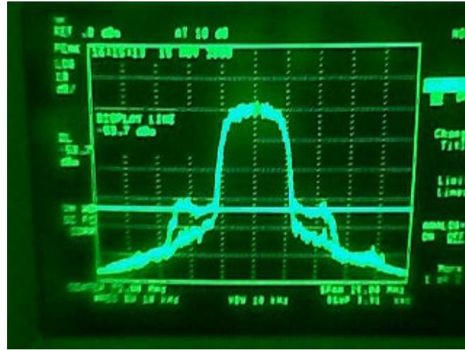
Figure 5.16: Spectrum of PA Output Using Predistortion at Low Input Power
