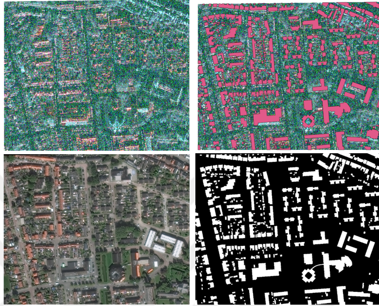
Figure 5.2: Dataset examples: Top row shows SAR images. The bottom left shows optical images of the same tile, and the bottom right shows ground truth.
