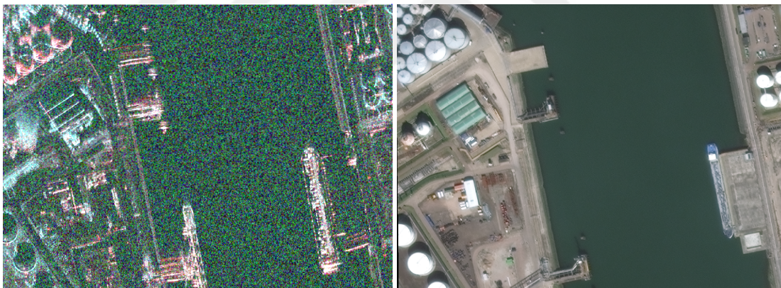
Figure 3.1: Comparison of SAR image with Electro Optic image
