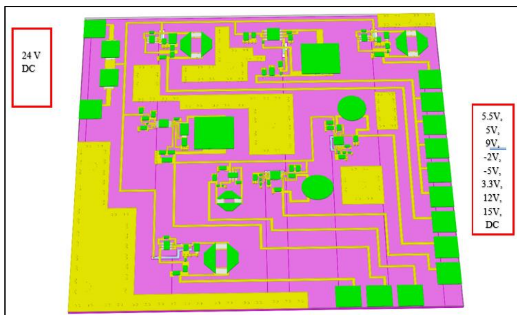
Figure 3.109. 24V input voltage and DC voltage outputs
