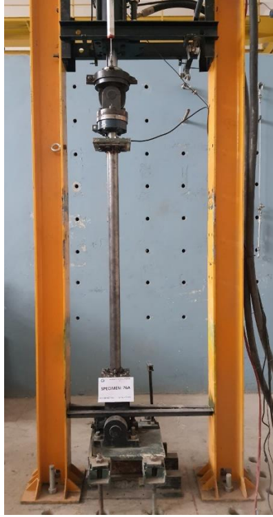
Figure 22. Specimen 76A ready for test
