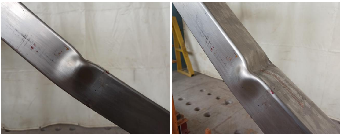
Figure 1. Local buckling (Demir et al., 2024)
