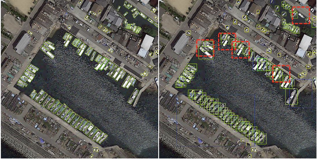
Figure 4.11: Ship detection difference between horizontal and oriented detectors in condensed setting.
