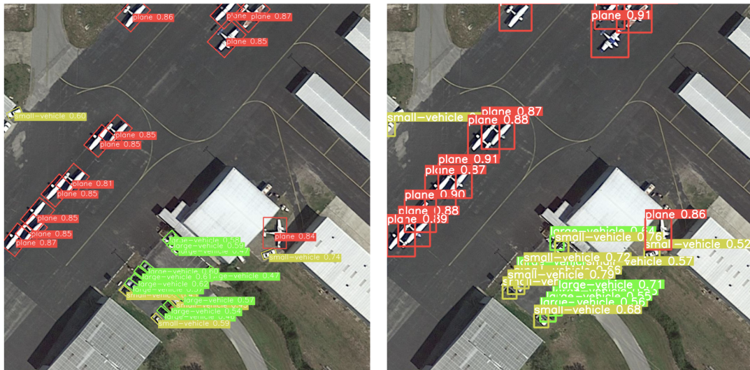
Figure 4.9: Fine grained class recognition problem in one-stage detection results.
