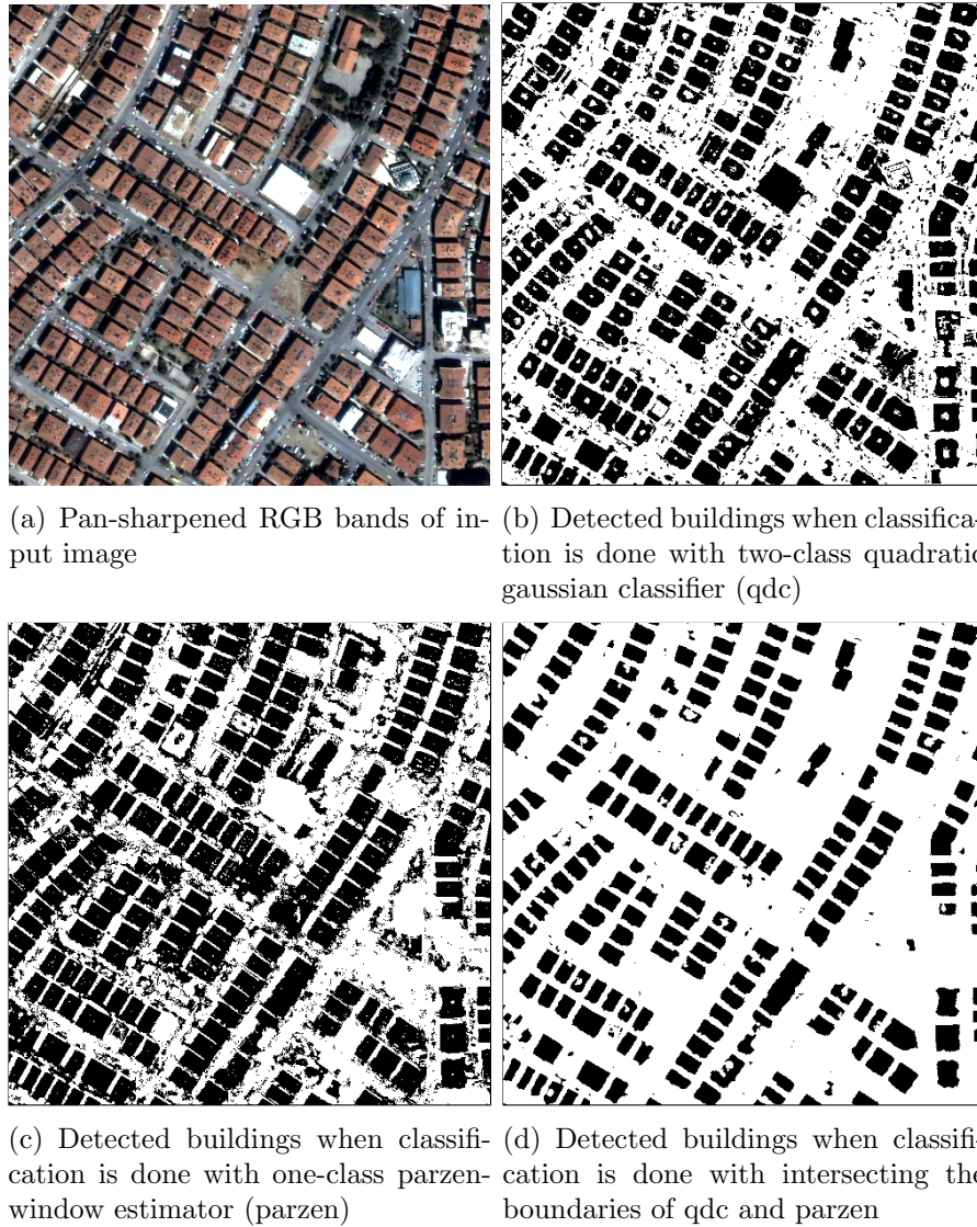
Figure 3.2: The use of combining different one-class and multi-class classifiers for better classification performance.
