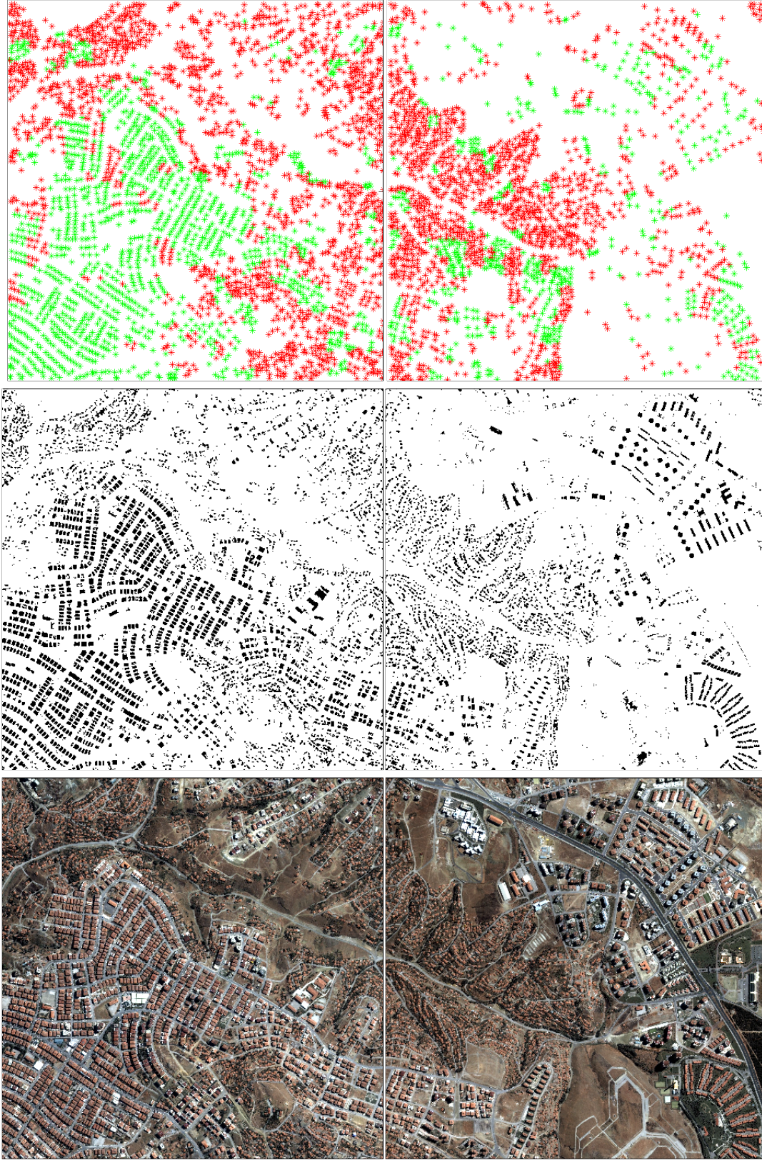
Figure 6.12: Example scene classification results for test images 1 and 2. The left column shows the original data, the middle column shows the detected buildings, and the right column shows the neighborhoods classified using the fourier domain features. Buildings that belong to neighborhoods classified as organized are shown as green and buildings in unorganized neighborhoods are shown in red.
