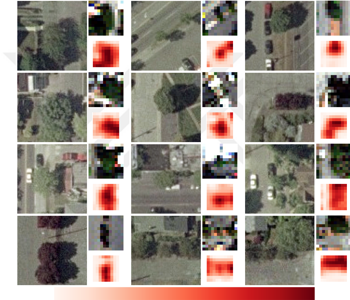
Figure 5.5: Weights of region proposals estimated from randomly selected 12 multispectral test images. For each sample, 25 \times 25 pixel RGB patch is shown on the left, the normalized RGB bands of the 12 \times 12 multispectral patch covering the same region with RGB patch is shown on top-right, and the weight distribution of region proposals is shown on bottom-right. Each weight value is the weight of a 4 \times 4 region proposal whose center pixel corresponds to the pixel of this weight value.
