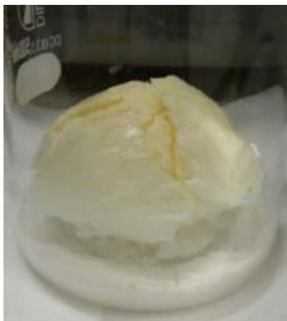
Figure 2.10. Strontium aluminate pre-ceramic material after dehydration at 120°C for 24 hours.
