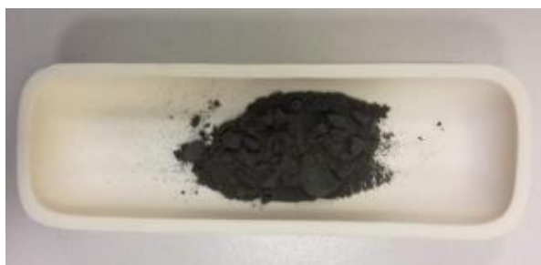
Figure 2.11. Strontium aluminate compounds after organics burn out by pre-calcination at 600 °C for 6h and then 700°C for 2h.
