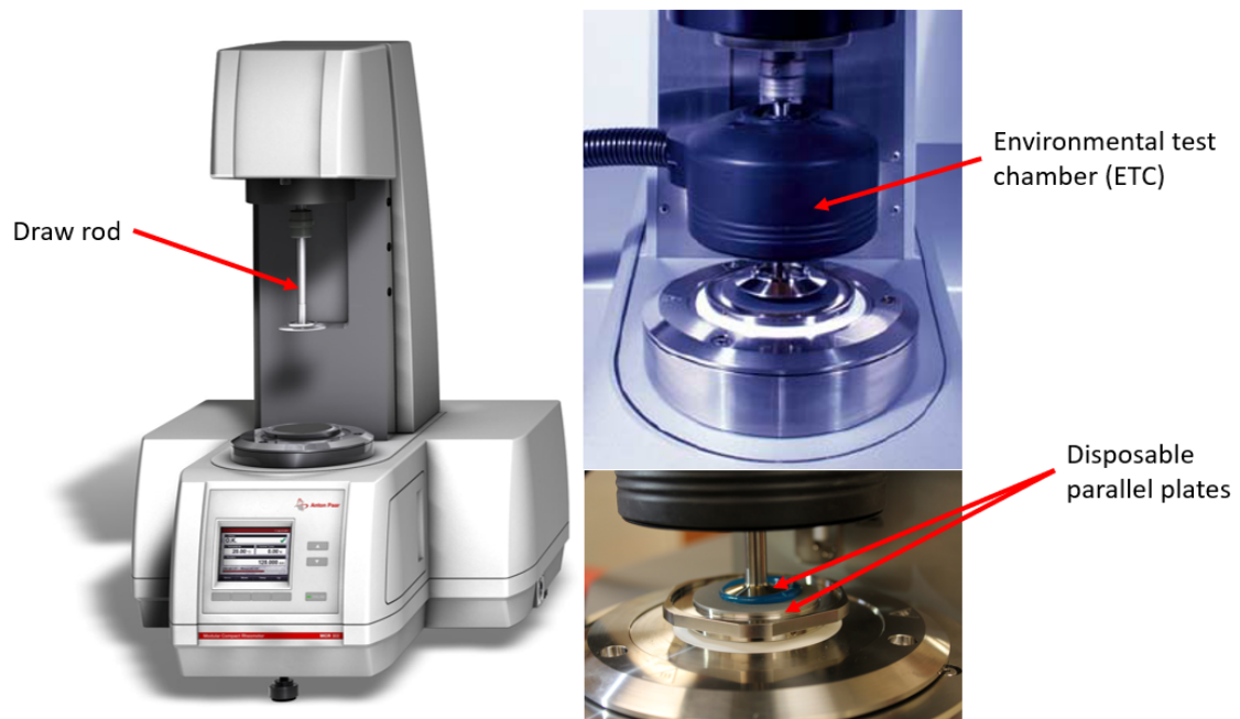
Figure 2.8 Rheometer (left); environmental test chamber (ETC) detailed view (right-top); close-up view of the Disposable parallel plates and the resin specimen (right-bottom) [57]
