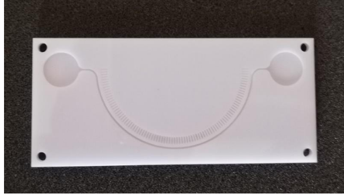
Figure 5.2 The semicircular microchannel unit with white ground color (Personal archive, 2019)
