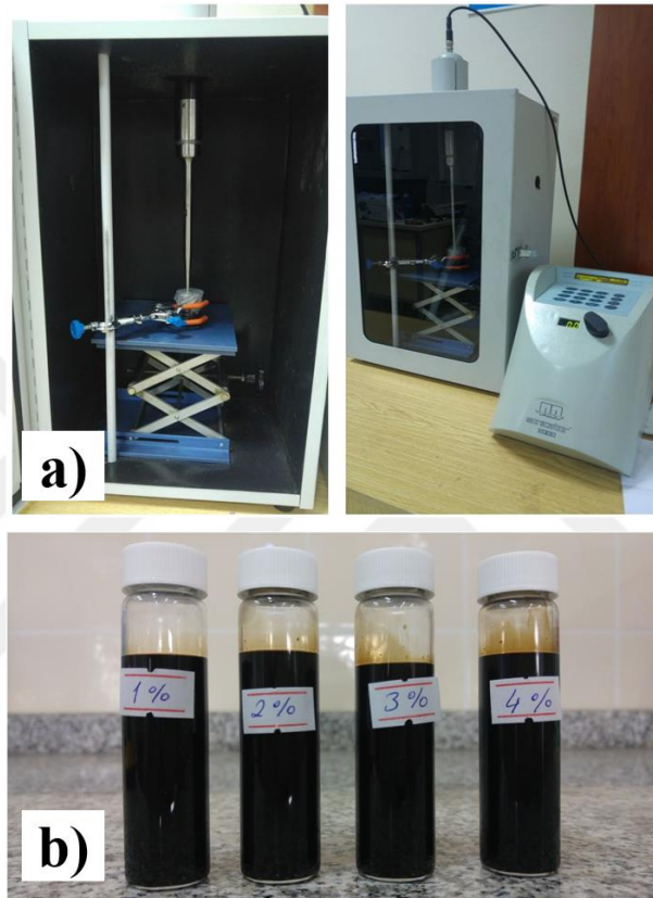
Figure 2.1 (a) Probe type Misonix Sonicator 3000 model ultrasonicator, (b) Images of the diluted and ultrasonicated Fe 3 O 4 samples (Personal archive, 2018)
