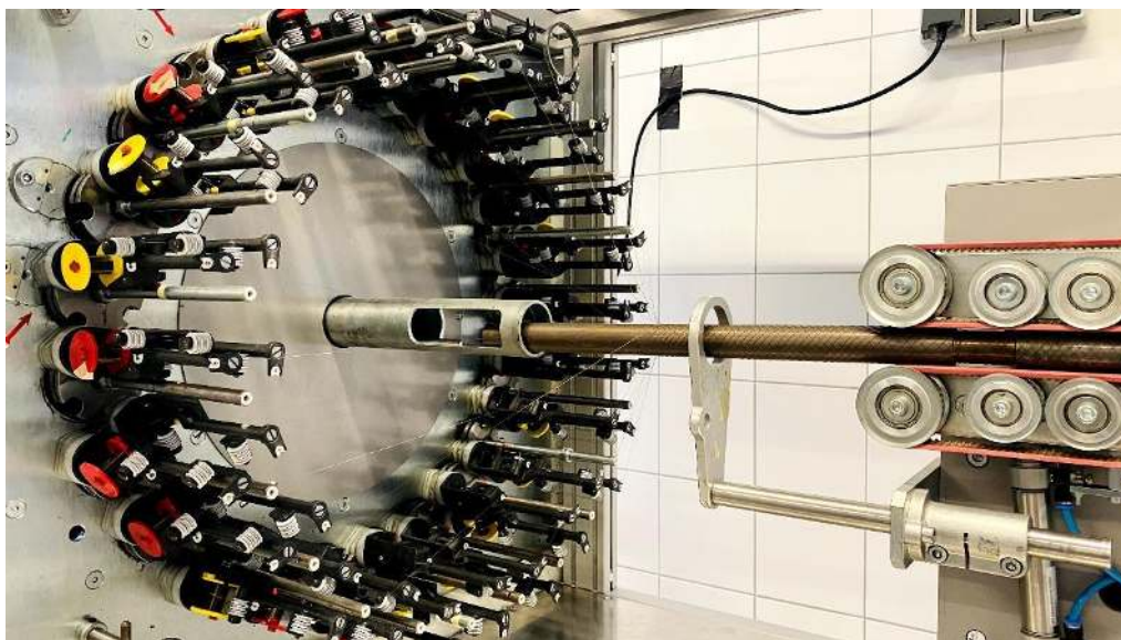
Figure 3.6. Steeger braiding machine for producing stents
