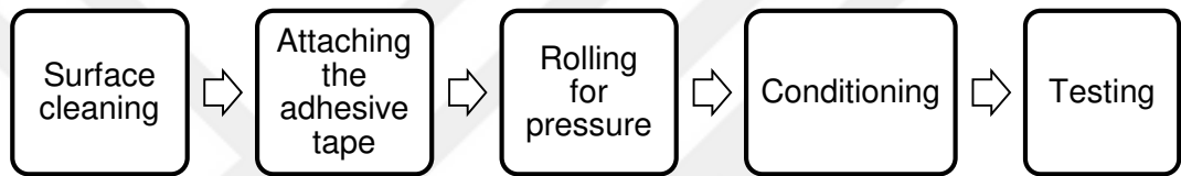
Figure 3.3. Flowchart of sample preparation for 2D samples
