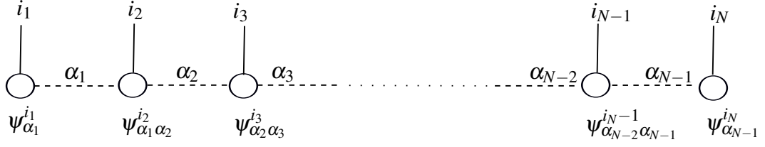
Figure 2.2: Graphical representation of MPS where the circles indicate the tensors associated with each site. The number of the legs for each site is equal to the number of indices of the related tensor.
