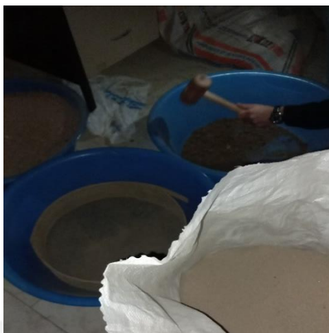
Crushing the soil sample with a wooden hammer
