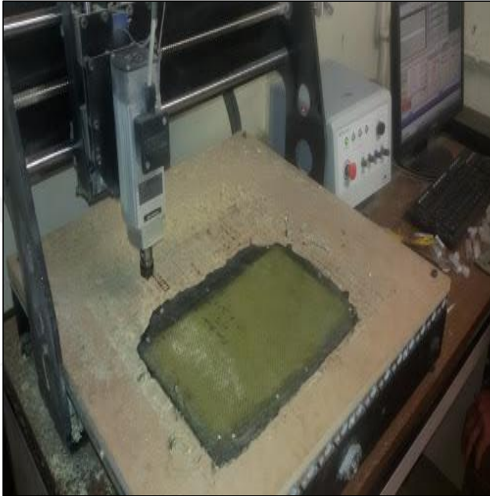
Figure 3.10 Cutting the specimen using CNC
