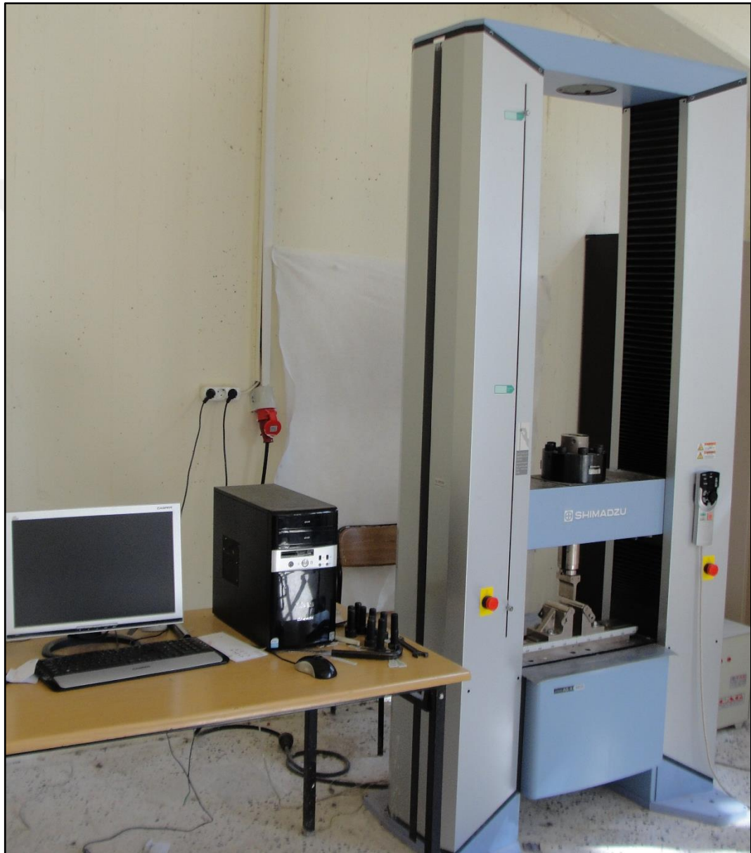
Figure 3.12 Test set-up Shimadzu AG-X series testing machine
