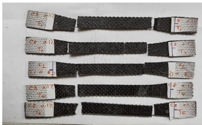
Figure 4. 19 samples of carbon fiber epoxy graphene composite after failure
