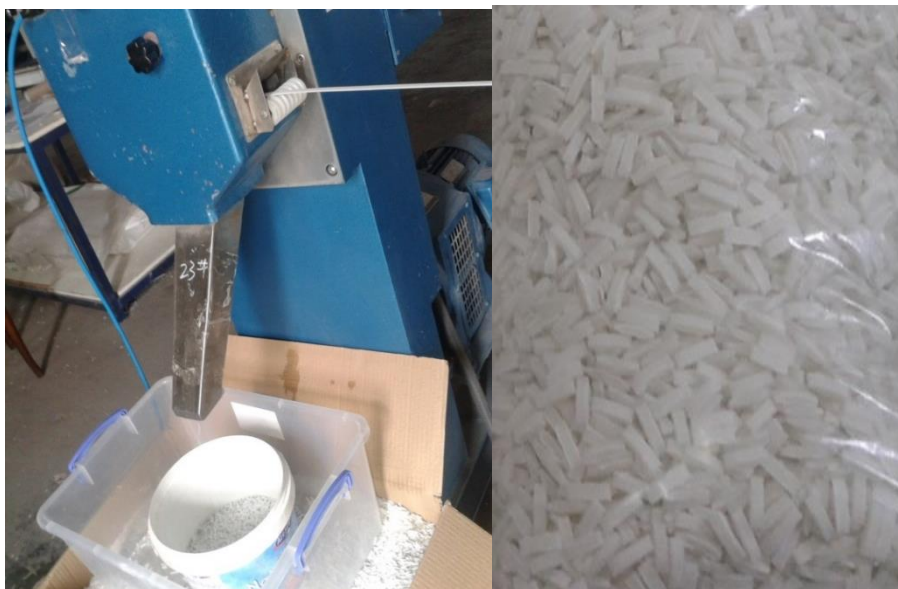
Figure 5.1 Pelletizing of R-PET/HDPE Blend and granules.
