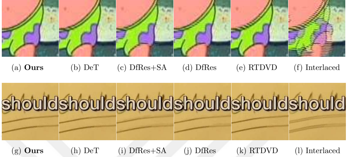
Figure 5.6: Deinterlacing results on real-world data. (f) and (l) are interlaced frames, where even and odd fields are weaved. (a)-(e) and (g)-(k) are deinterlaced results for the bottom field of the corresponding interlaced frames.
