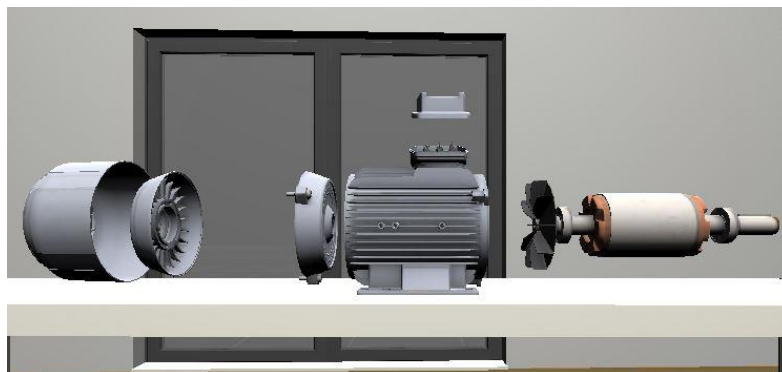
Figure 6.25. Removing stator cover from the stator.
