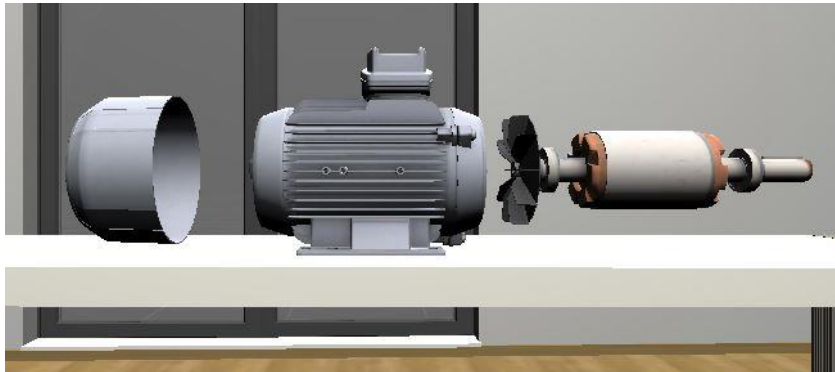
Figure 6.23. Removing rotor from the stator.
