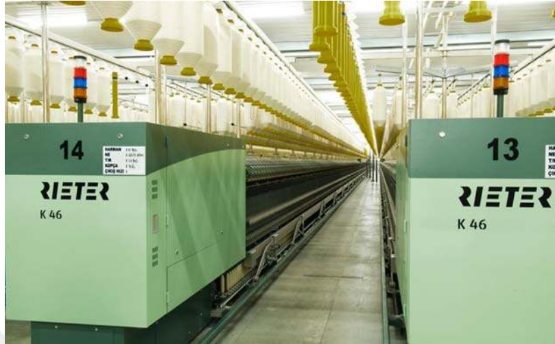
Figure 1.3. Compact machine (Rieter k-46)
