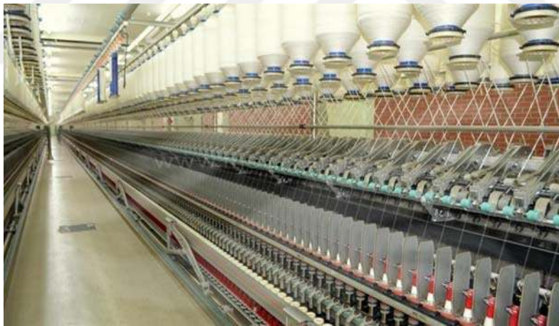
Figure 1.1. Ring spinning system
