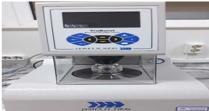
Figure 3.6. The bursting strength tester
