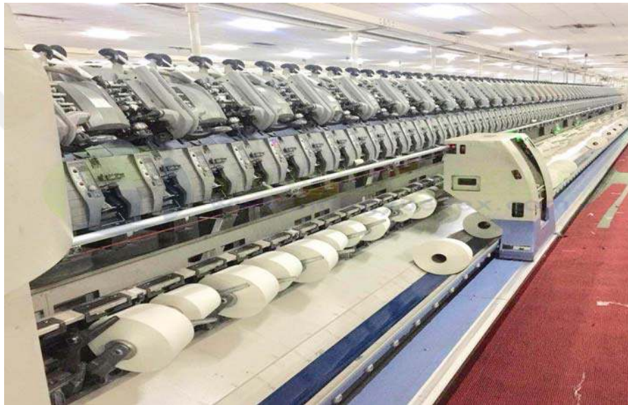
Figure 1.5. Vortex machine (MVS III 870)
