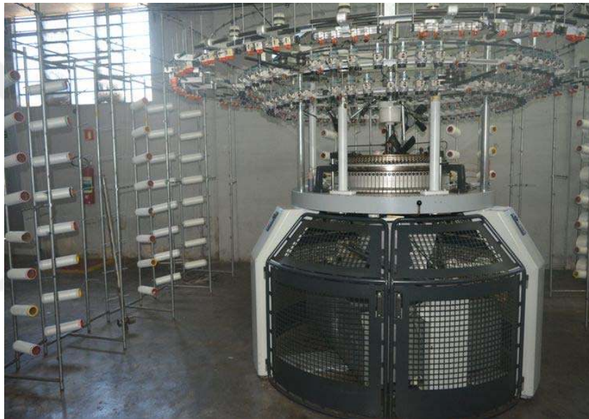
Figure 3.3. Knitting machine Mayer &amp; Cie MV 4 32"
