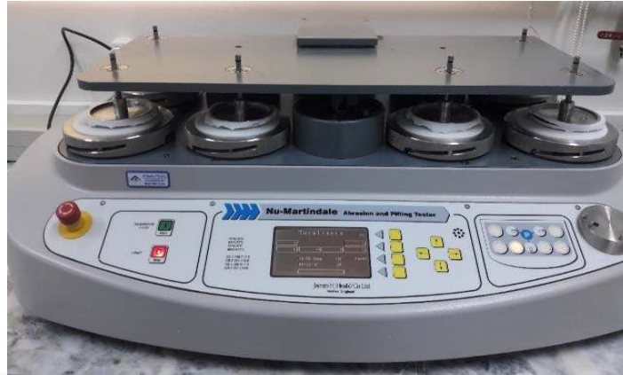
Figure 3.4. Nu-Martindale abrasion and pilling tester
