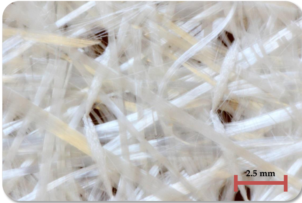
Figure 2-1. Fibroteks E-glass Stitched Random Fabric.
