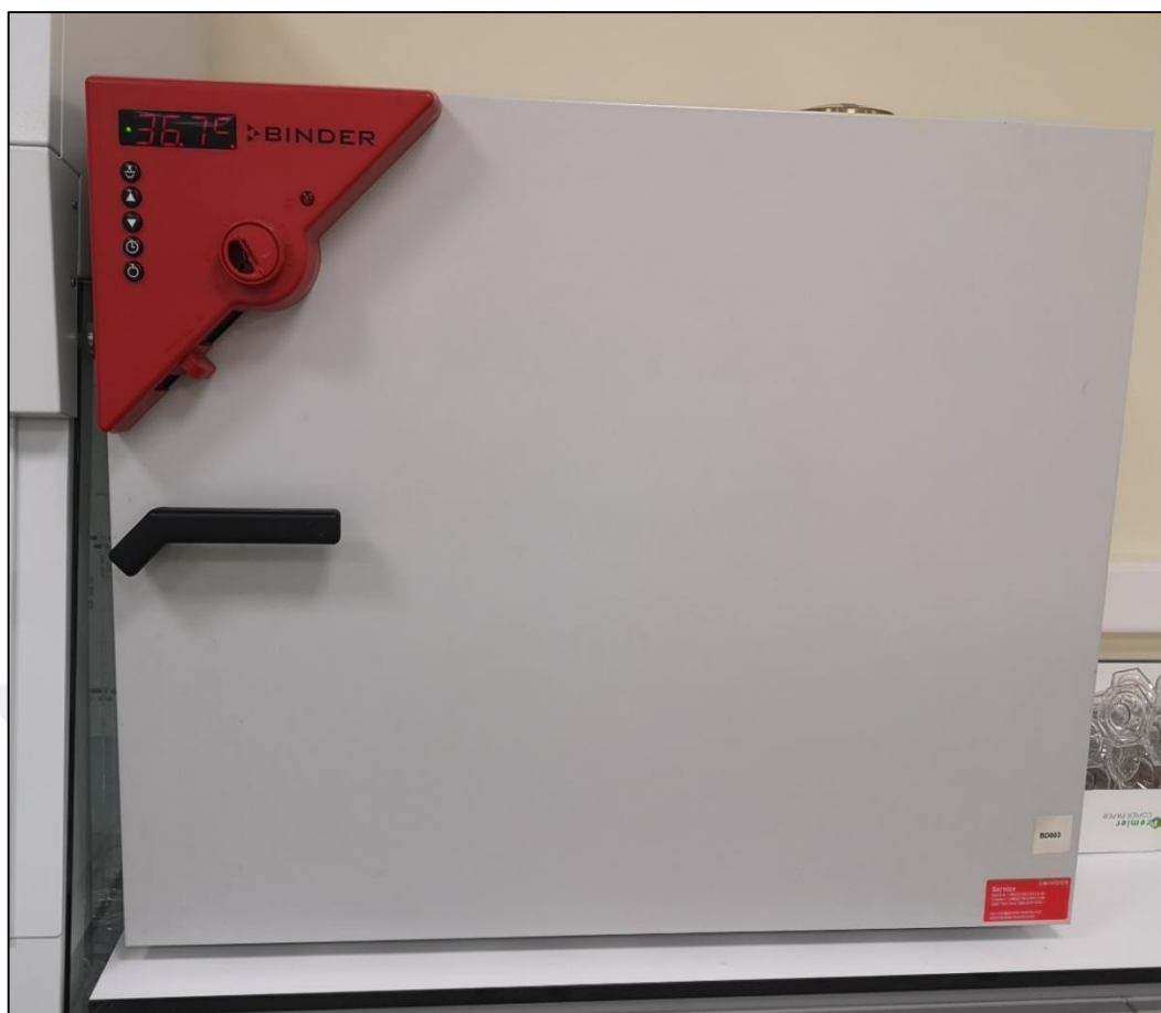
Fig.13. The incubator which provides storage of the samples at 37°C
