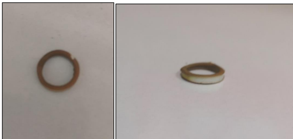
Fig.10. Polyvinyl chloride molds with a diameter of 8.0±0.1 mm and a thickness of 1.6±0.1 mm
