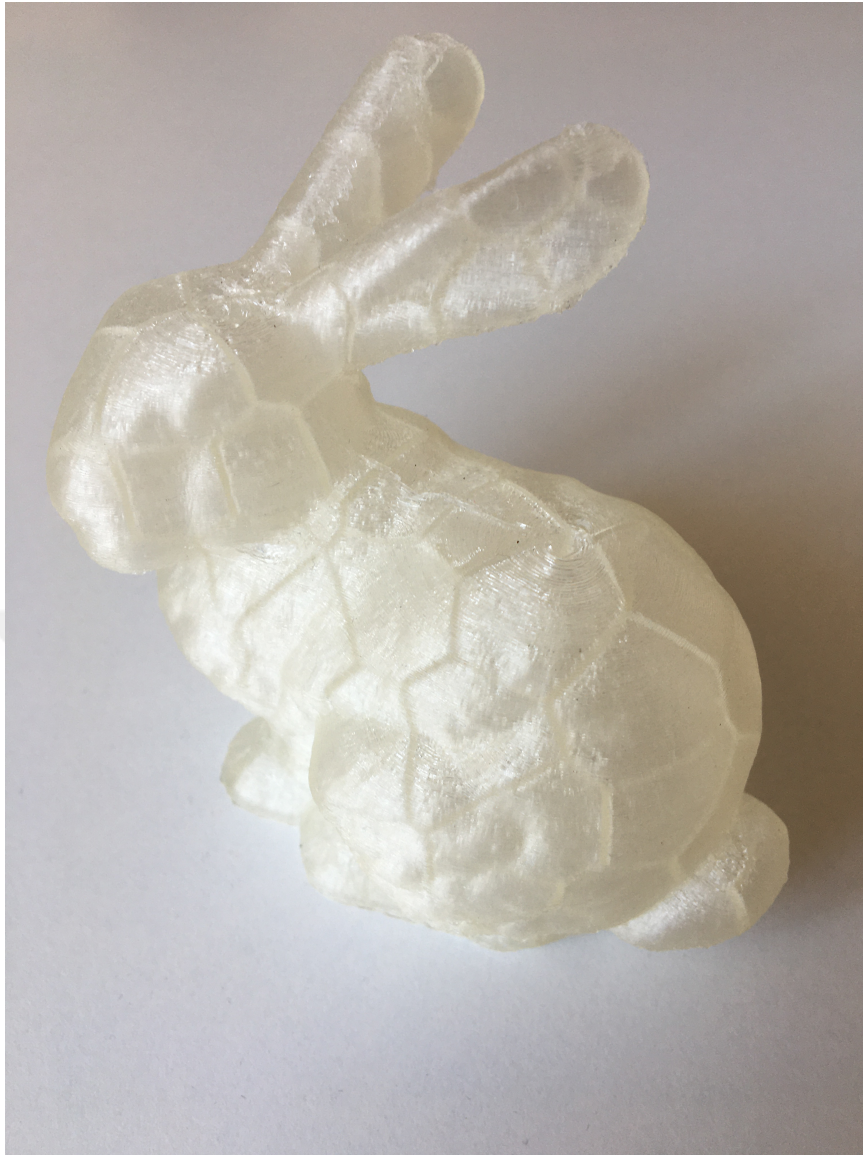
Figure 4.30: Bunny with 100 Voronois and 1 layer of shell, 3D printed with transparent filament.
