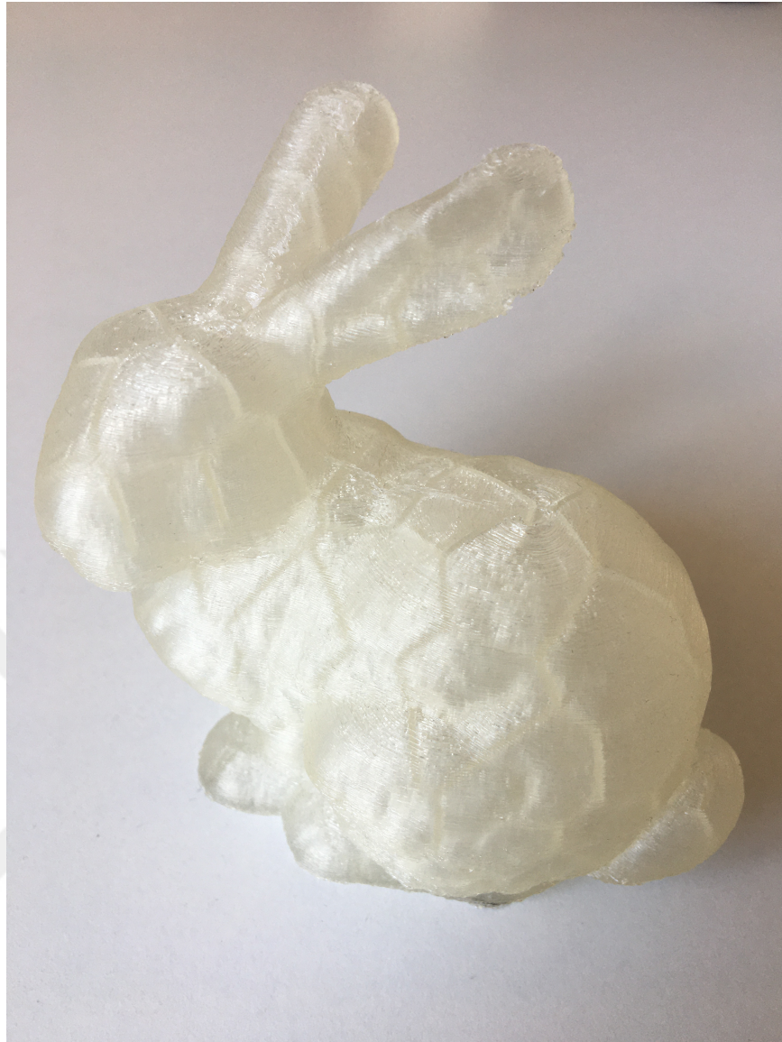
Figure 4.29: Bunny with 100 Voronois and 2 layers of shell, 3D printed with transparent filament.
