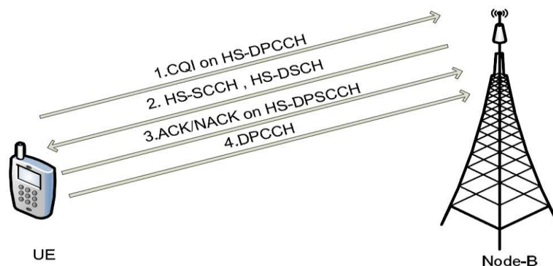
Figure 3.9 Transmission method in HSDPA
