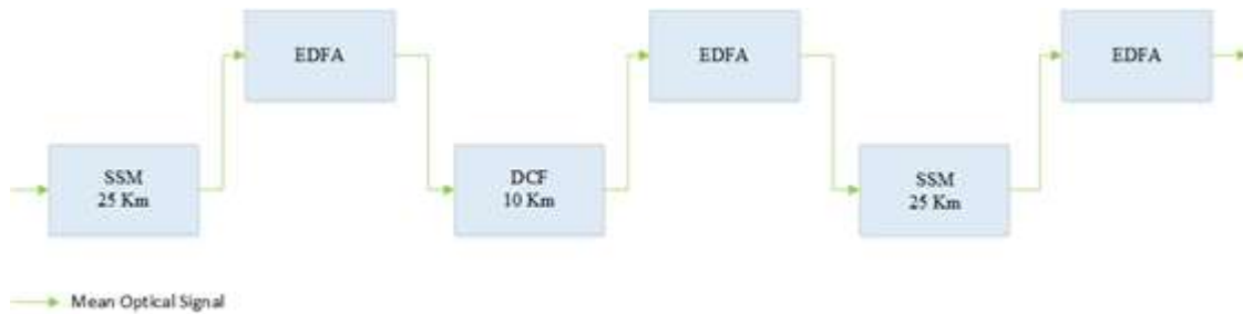
Figure (4.2): Transmission link components
