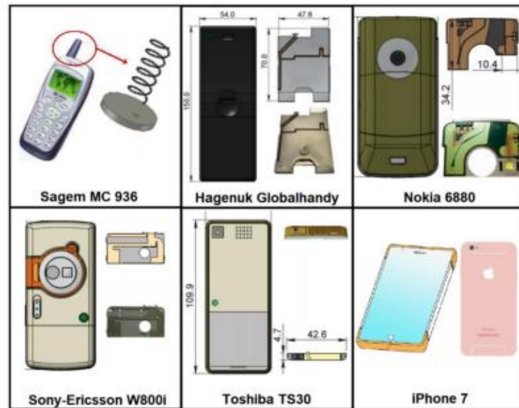
Figure 1.6 The various varieties of antennas utilized by mobile phones.
