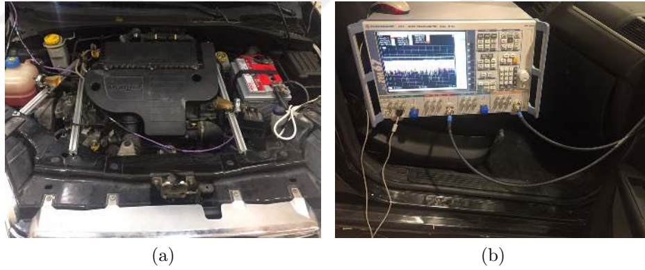
Figure 3.2: Measurement setup (a) Transmitter (Tx) and receiver (Rx) antennas in the engine compartment of Fiat Linea, (b) VNA connection to the antennas.
