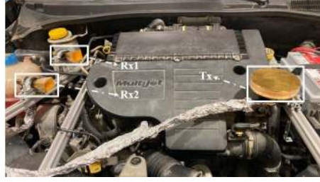
Figure 6.2: Transmitter and receiver antennas in the engine compartment.
