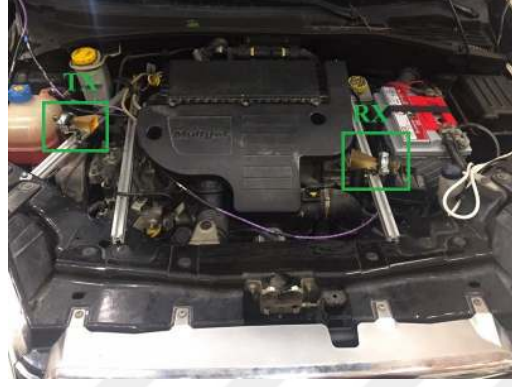
Figure 2.2: Transmitter and receiver antennas in the engine compartment.
