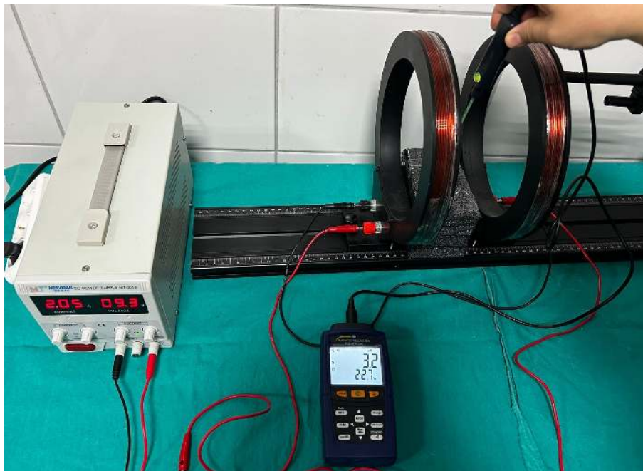
Figure 4.4 : Measurement of static magnetic fields utilizing Helmholtz coils with Gaussmeter.
