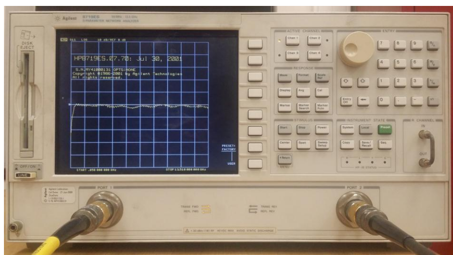
Figure 5.4: Agilent HP8719ES Network Analyzer (0.05-13.5GHz).
