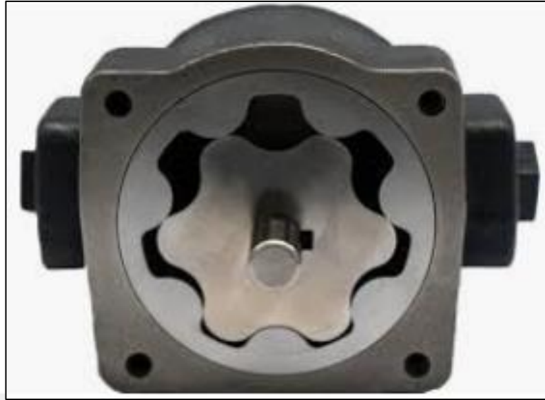
Figure 3.16 Schematic view of ge-rotor pump (Gerotor Design Study, 2018)
