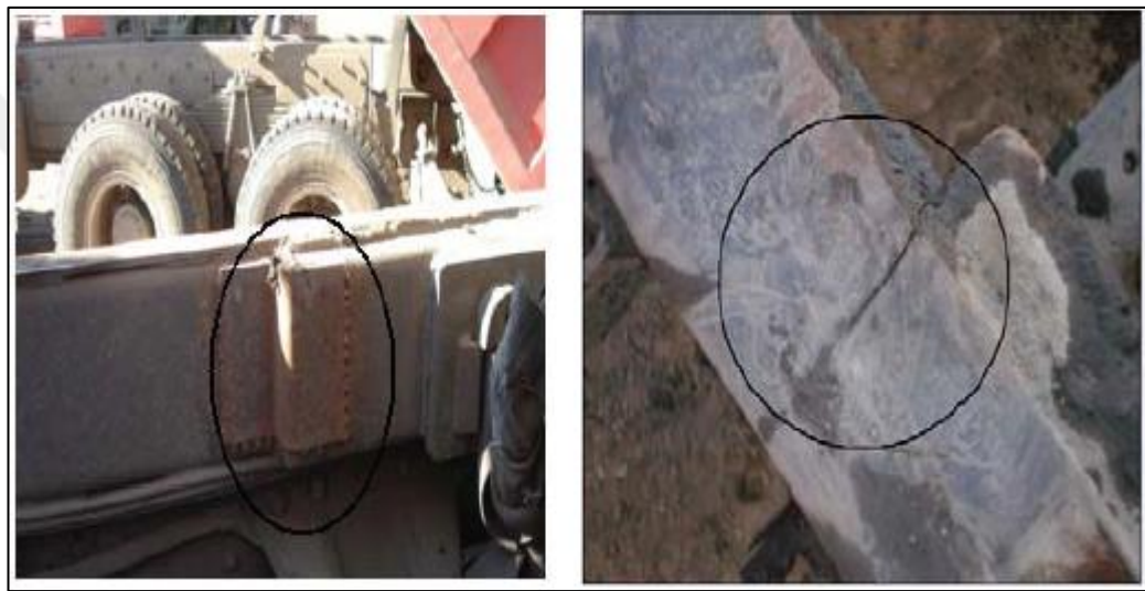
Figure 2.1 The fatigue crack of the sub-frame (Yanhong, & Feng, 2011)
