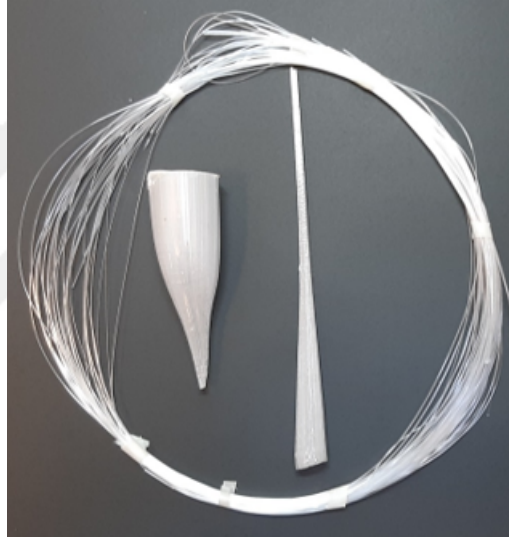
Figure 4.3: Collected thermally drawn HCMPOF ( \sim 10\text{m} ) with preform ends.
