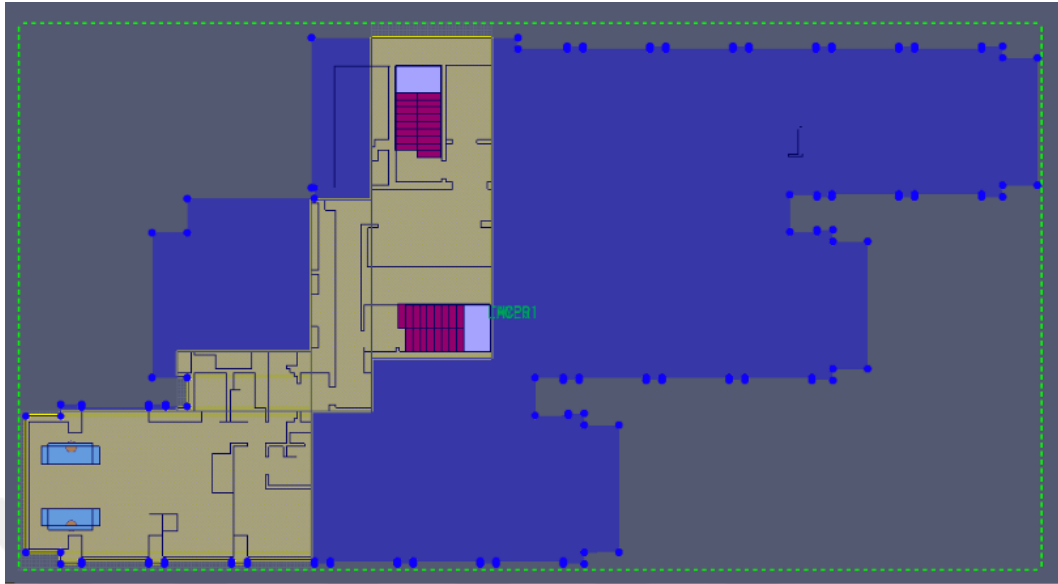
Figure B.2. PyroSim fire model of representative building.
