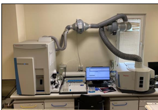
(e) IMS-CP used for cation release testing
