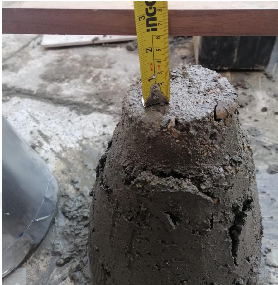
Figure 3.4: The Concrete Slump Test.
