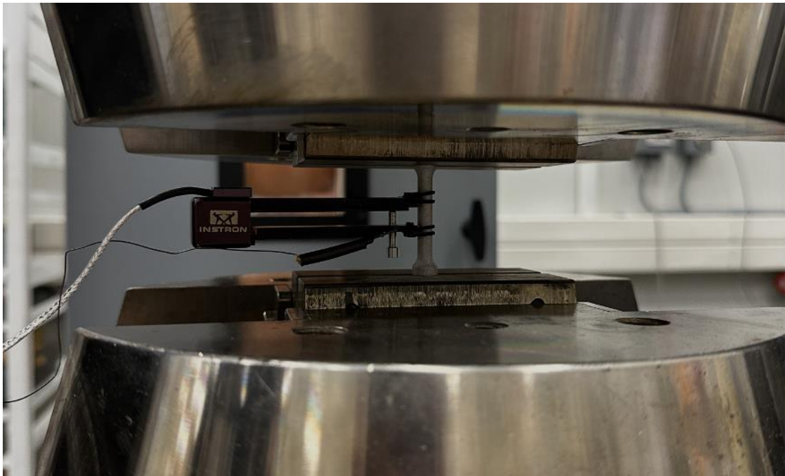
Figure 5.2 Tensile test of samples with extensometer
