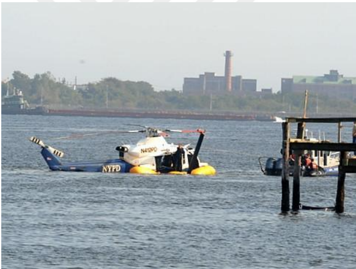
Figure 3.5 The Bell 412EP helicopter resting in Jamaica Bay after the emergency landing [210].
