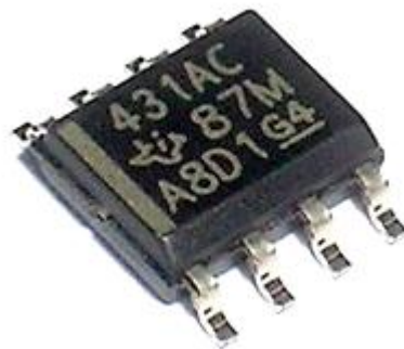
Figure 2.29 TL431 in SO8 surface mount package
