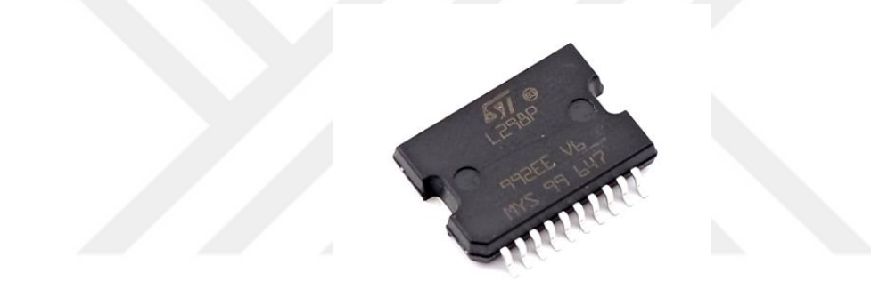
Figure 2.55 Outlook of “PowerSO20” SMD package of L298
