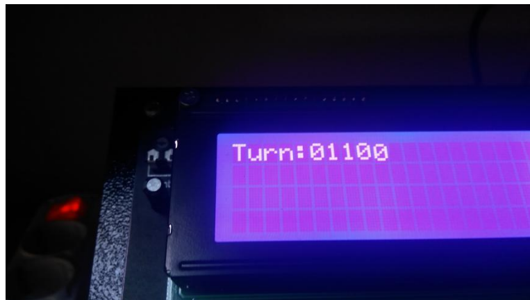
Figure 2.11 Winding turns counter (Personal archive, 2019)
