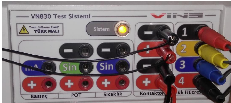
Figure 2.16 VN830 data acquisition and analysis system (Personal archive, 2019)
