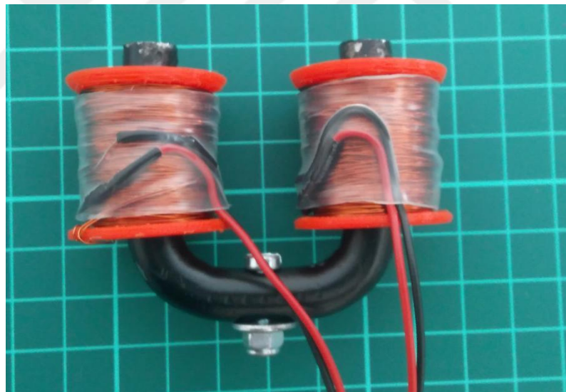
Figure 2.13 Finished electromagnet (Personal archive, 2019)
