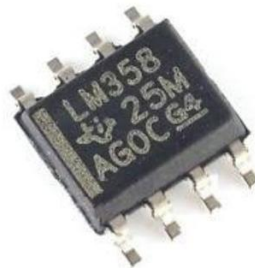
Figure 2.32 LM358 Opamp in SO8 package
