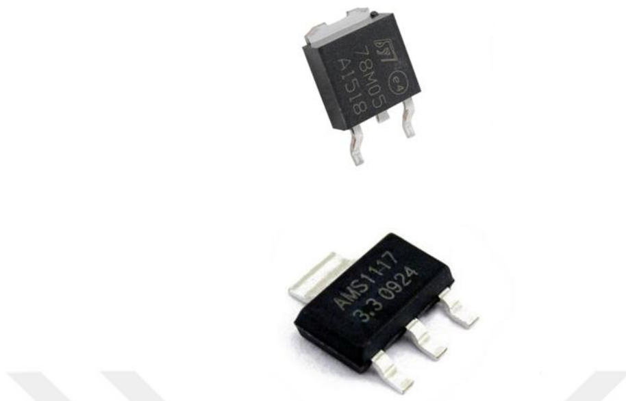
Figure 2.27 78M05 and AMS1117-3.3 IC in SMD packages
